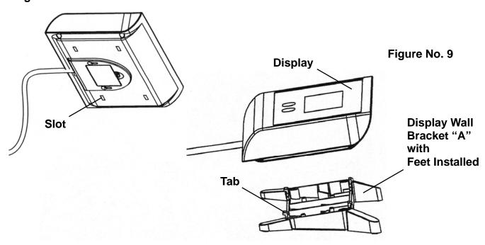
4. Referring to Figure No. 9, align and insert the tabs on the bracket with the slots in the display back and press together until the bracket locks to the back of the display.
